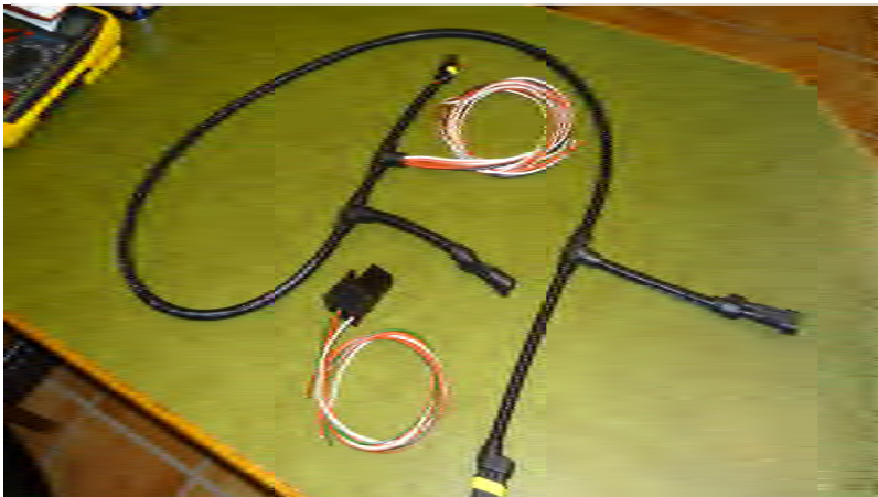
Completed Main Harness including micro relay assembly for DRL Control.
