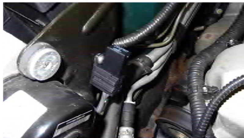
New 5 pin changeover Micro Relay fitted in base to side of ABS motor bracket.
