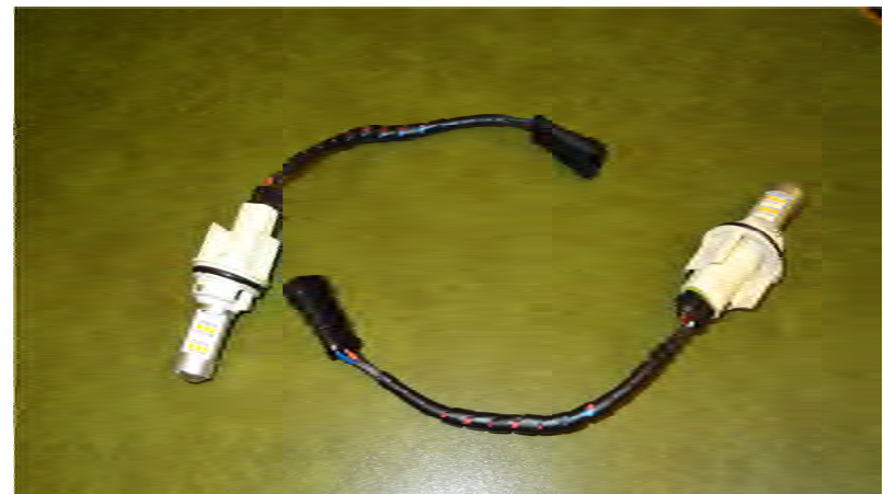
Modified DRL/Turn Switchback lamps with new harnesses.
