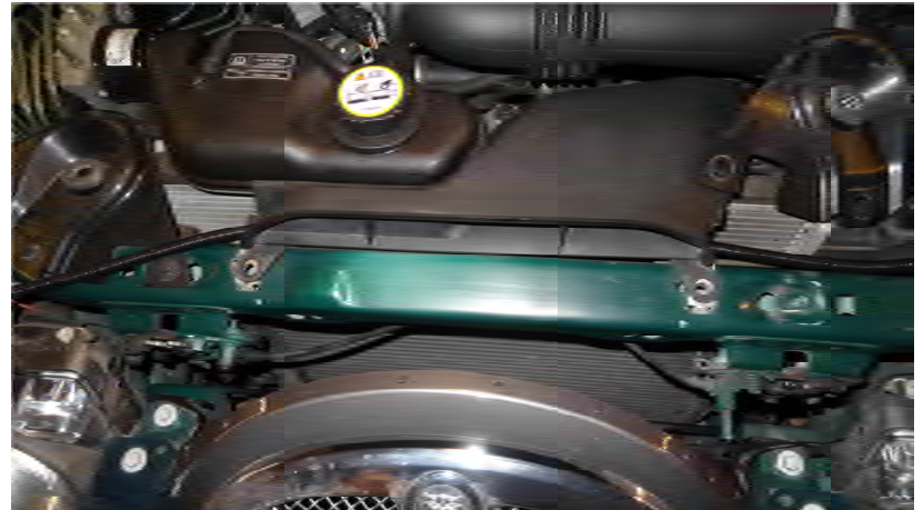
Pass main harness underneath air intake and both top radiator mountings.
