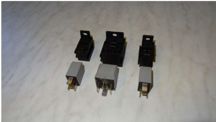
Three relays with interlocking bases. One for each turn signal LED and one for White switchback control..
