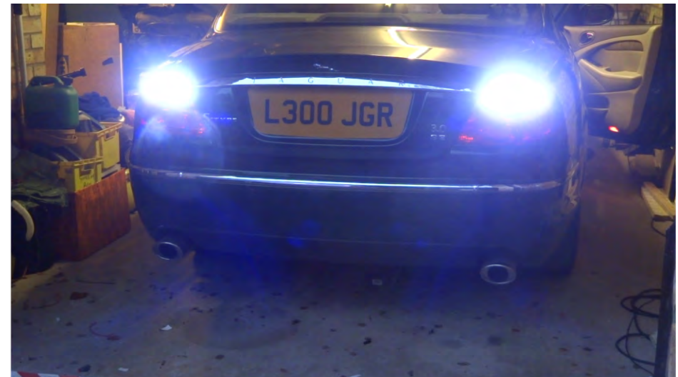
Reverse Gear Selected New Switchback White LEDs and 100W 1156 Reverse LED bulbs
