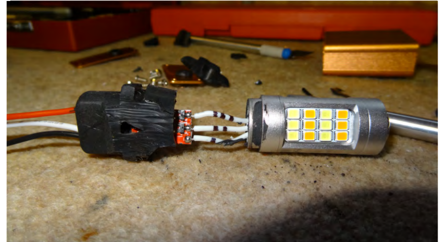
Carefully cut away the rubber which houses the switchback circuit board as shown. Use a very sharp scalpel type knife being careful not to damage or cause undue strain on the circuit board and wires. Mark each wire with black marker as shown and then unsolder the connections. Cut away rubber housing as shown as this will fit snugly into the aluminium housing.
