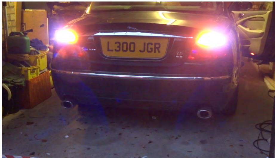
Hazards and Reverse Gear Selected New Switchback Turn LEDs and 100W 1156 Reverse LED bulbs
