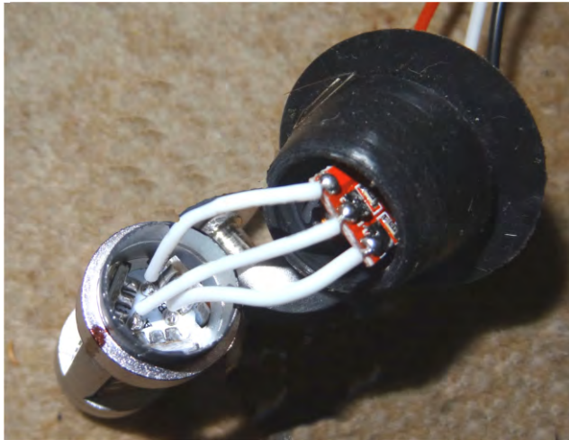
Carefully separate the lamp from the rubber circuit board housing. The lamp and PCB are fixed with black silicon sealer. The solder connections are fragile.
